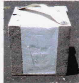
Solarcrete's energy-efficient wall consists of a foam core between two layers of concrete
